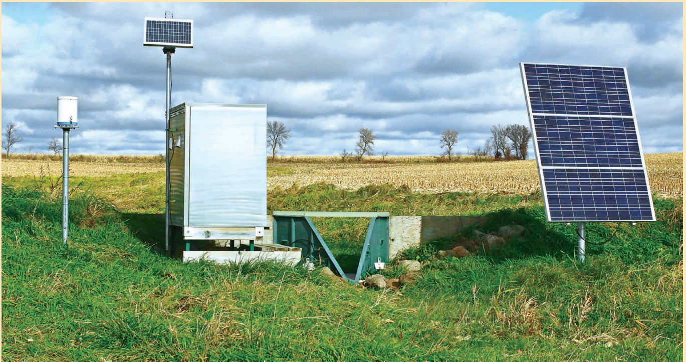
An edge-of-field runoff monitoring station in the Dry Run watershed.
