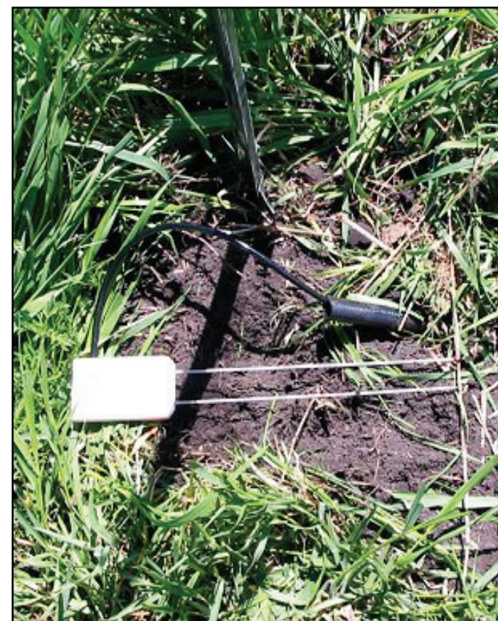
Figure 6. Campbell Scientific CS616 soil moisture probe
