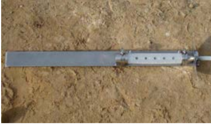
Figure 30: Sample line strainer attached to steel plate.
