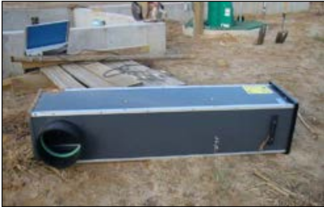
Figure 33: Agri Drain to measure flow in pipe.
