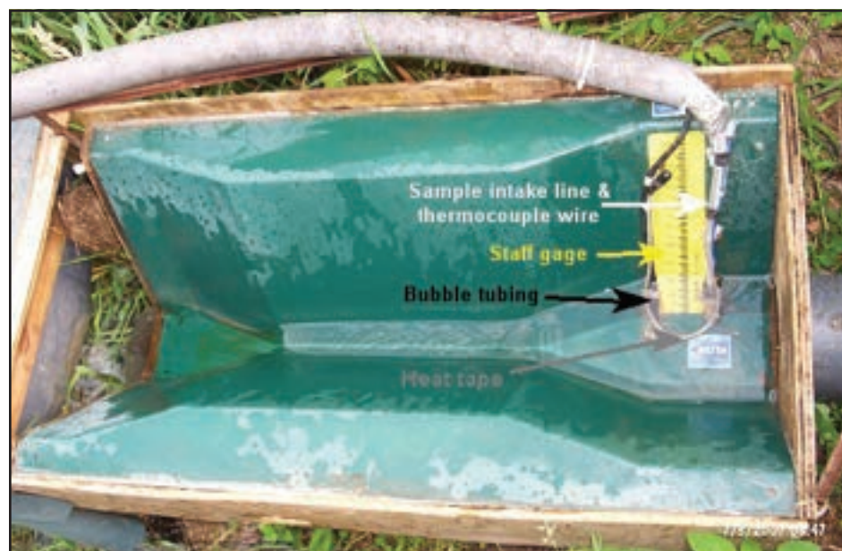
Figure 5. Trapezoidal flume, lines, thermocouple wire & heat tape
