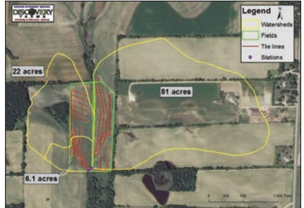
Figure 2. Monitored fields with contributing areas (yellow) and tile line schematic (red)
