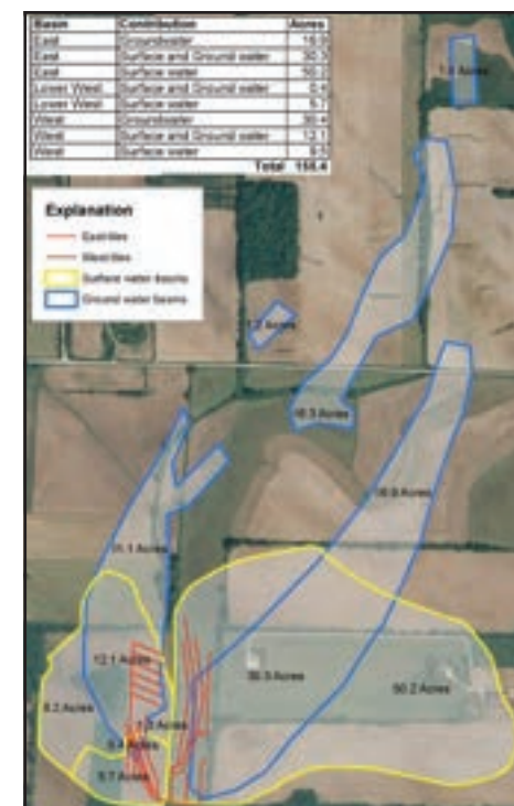
Figure 20. Basin contributing areas defined by surface topography (yellow) and groundwater modeling (blue) to tile drainage system (red).
